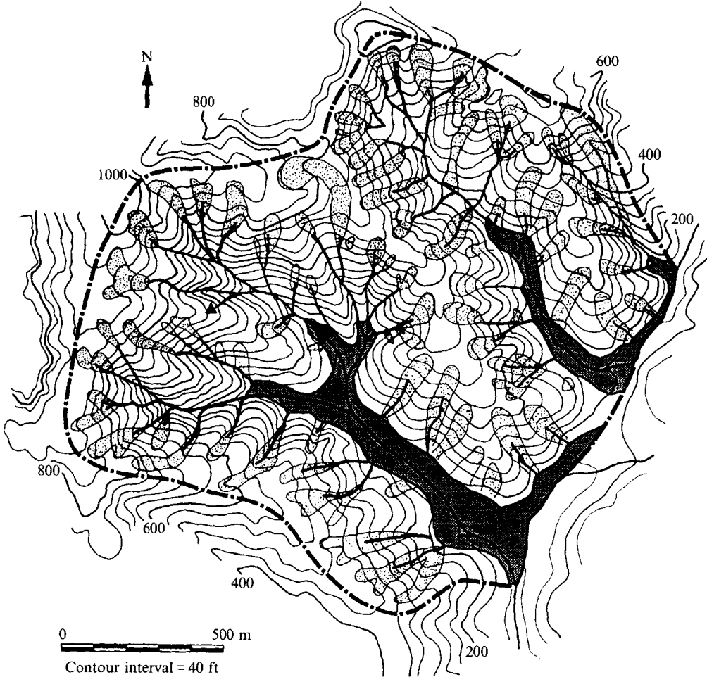
FIGURE 1. Map of the channel network (heavy solid lines), areas of thick colluvium (stippled area) and thick valley floor deposits of colluvium and alluvium (shaded area) near the headwaters of the Tennessee Valley drainage basin of Marin County, California. (Courtesy W. E. Dietrich; from Dietrich et al. 1993).
